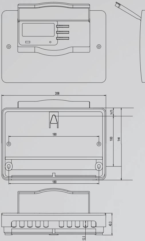
**Housing:** plastic, PC-ABS and PMMA
