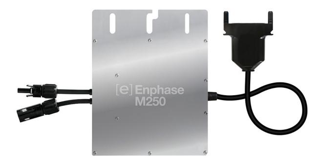
The **Enphase** M250 Microinverter delivers increased energy harvest and reduces design and installation complexity with its all-AC approach. With the M250, the DC circuit is isolated and insulated from ground, so **no Ground Electrode Conductor (GEC)** is required for the microinverter. This further simplifies installation, enhances safety, and saves on labor and materials costs.
